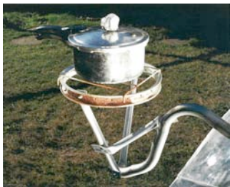
A gimbaled pot support made from 12" used bicycle rim attached to metal tubing.
