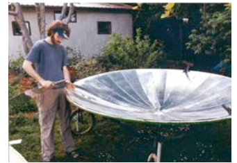
HSU student riveting aluminum to dish.
