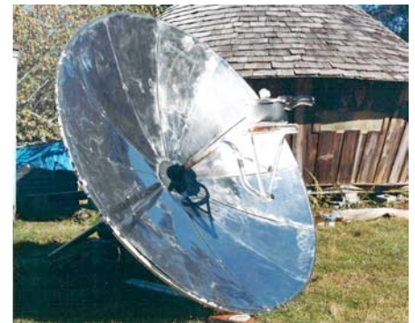
The pot support on this 6' stainless steel dish is attached to a piece of tubing coming up through the center of the dish.
