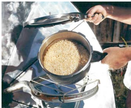
Brown rice cooked in 30 min in a pressure cooker on a parabolic dish.
